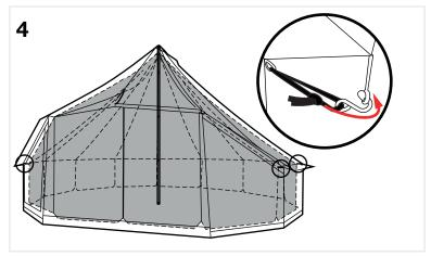
Attach the metal hooks to the corresponding O-ring of the tent and tighten the guylines.
