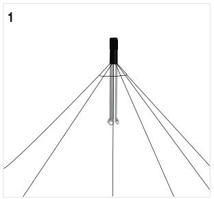
Release the tension on the guylines and remove the center pole. Unroll the inner liner and make sure that the D rings are positioned inside the tent. the center pole out of the tent.
