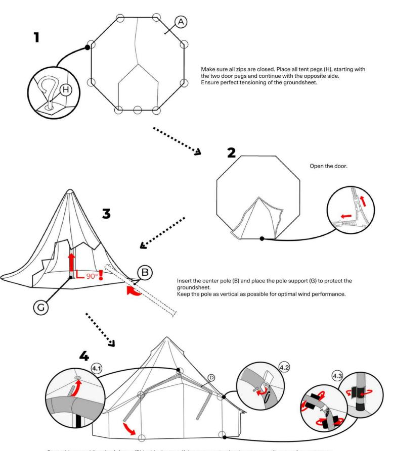
Start with assembling the A-frame (D) inside the tent. If there are protective rings surrounding your frame, remove them to avoid staining and damaging the fabric.
